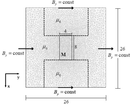
**Figure 1:** Domain geometry, mesh and boundary conditions for the magnetostatic problem. Dashed lines indicate the location of the nonmagnetic grips of the load frame.
