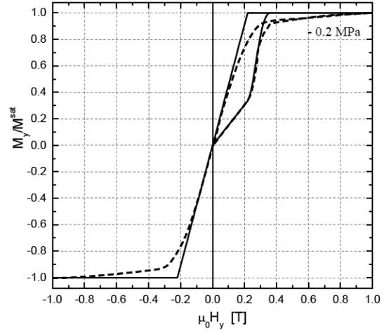
**Figure 6:** Predicted magnetization curve when accounting for magnetic domain wall motion at low magnetic field and stress levels. Solid lines: Model. Dashed line: Experimental data [2].
