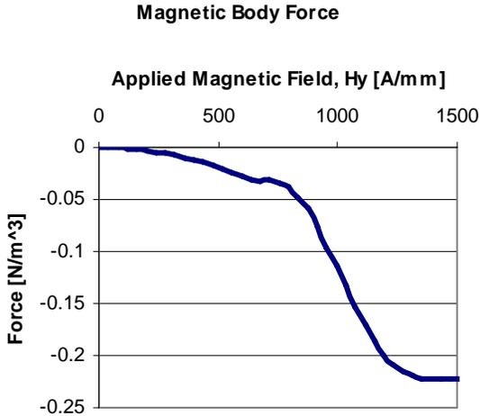
**Figure 2.** Maximum average magnetic body force magnitude as a function of the applied magnetic field.
