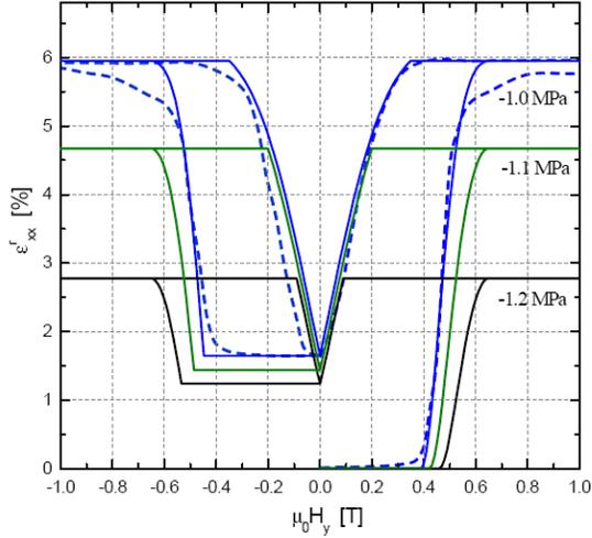
**Figure 3:** Predicted MFIS hysteresis curves at different stress levels. Solid lines: Model. Dashed lines: Experimental data [2].
