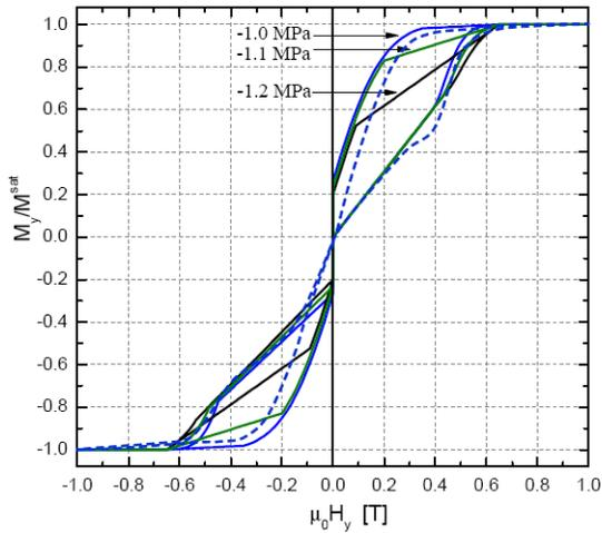
**Figure 4:** Predicted magnetization curves at different stress levels. Solid lines: model. Dashed line: experimental data [2].
