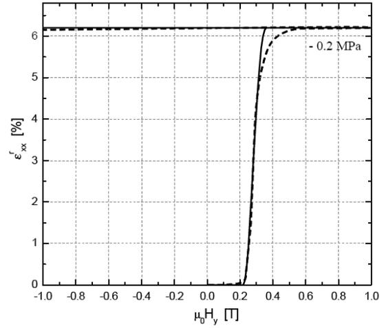
**Figure 5:** Predicted MFIS hysteresis curve. Solid Lines: Model. Dashed line: Experimental Data [2].
