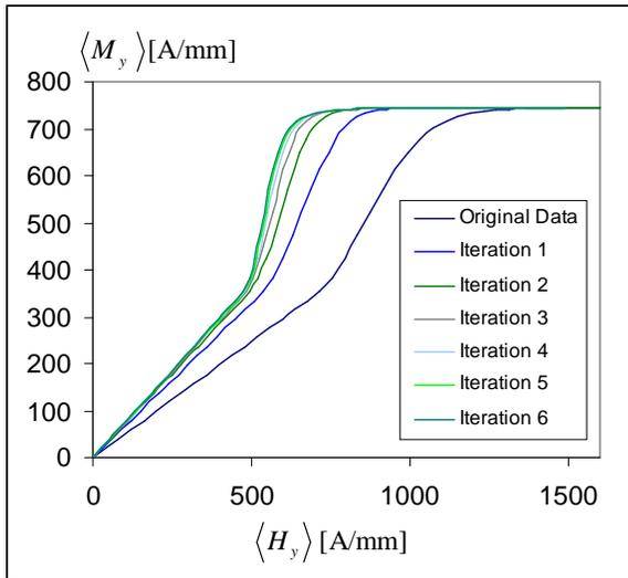
Figure 10. MAGNETIZATION DATA CORRECTED FOR DEMAGNETIZATION. SPECIMEN ASPECT RATIO 2:1.
