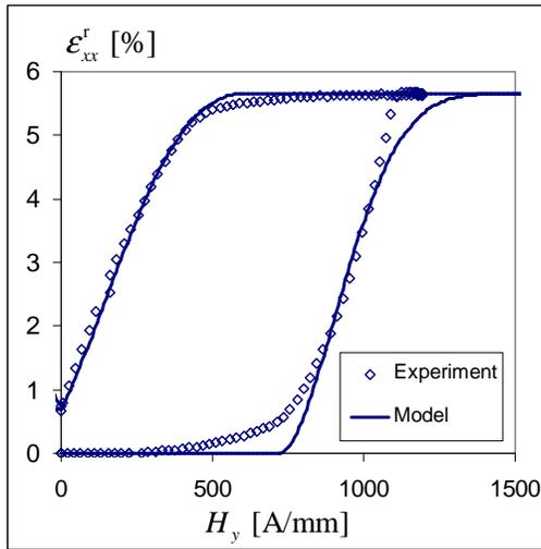
Figure 6. MODEL CALIBRATION. EXPERIMENTAL DATA (DIAMONDS) AND MODEL SIMULATION (SOLID LINE). DATA TAKEN FROM [23] FOR A  $\text{Ni}_{51.1}\text{Mn}_{24.0}\text{Ga}_{24.9}$  ALLOY TESTED AT  $-95^\circ\text{C}$  UNDER THE COMPRESSIVE STRESS OF 2 MPa.
