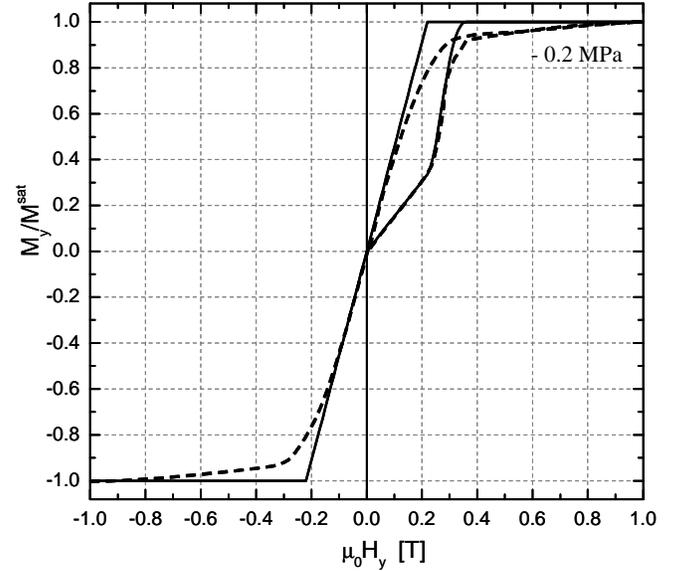
Figure 4. PREDICTED MAGNETIZATION CURVE WHEN ACCOUNTING FOR MAGNETIC DOMAIN WALL MOTION AT LOW MAGNETIC FIELD AND STRESS LEVELS. SOLID LINES: MODEL, DASHED LINE: EXPERIMENTAL DATA [2].
