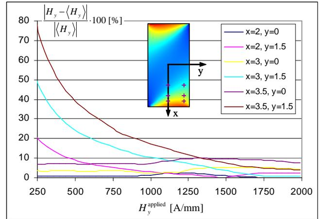
Figure 11. RELATIVE DIFFERENCE IN LOCAL AND AVERAGE  $H_y$  AT DIFFERENT LOCATIONS OF THE SPECIMEN VS. APPLIED MAGNETIC FIELD.
