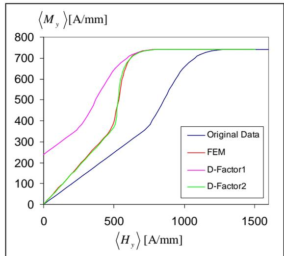
Figure 12. COMPARISON OF THE CORRECTIONS THROUGH DEMAGNETIZATION FACTORS AND FEM ANALYSIS. SPECIMEN ASPECT RATIO 2:1.
