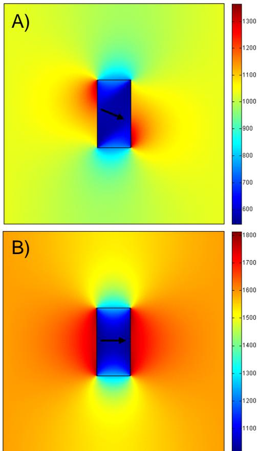
Figure 8. DISTRIBUTION OF  $H_y$  IN THE COMPUTATIONAL DOMAIN AN APPLIED MAGNETIC FLUX DENSITY OF A) 1.3 T, B) 2.0 T. (OR IN FIELD STRENGTH: A) 1034.5 A/mm, B) 1591.6 A/mm).
