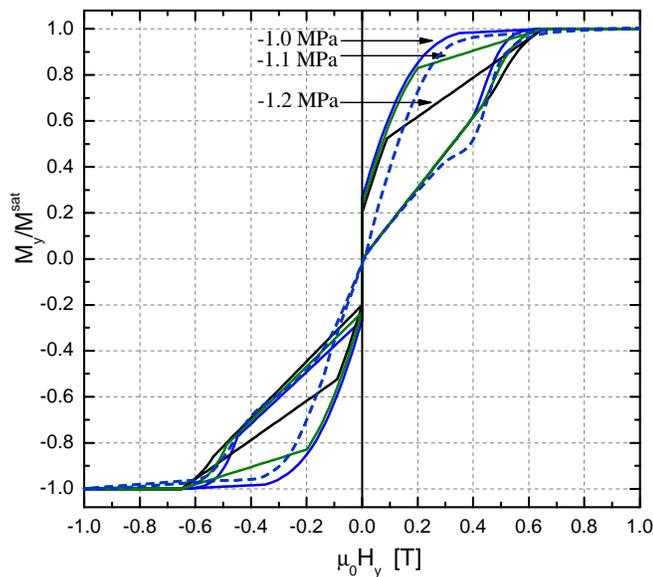
Figure 2. PREDICTED MAGNETIZATION CURVES AT DIFFERENT STRESS LEVELS. SOLID LINES: MODEL, DASHED LINE: EXPERIMENTAL DATA [2].
