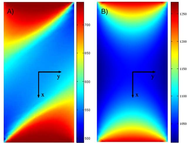
Figure 9. DISTRIBUTION OF  $H_y$  WITHIN THE SPECIMEN AT AN APPLIED MAGNETIC FLUX DENSITY OF A) 1.3 T AND B) 2.0 T.
