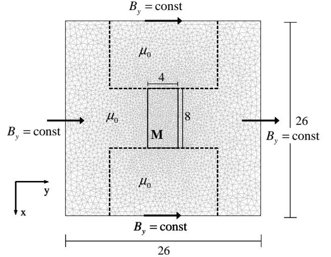
Figure 5. DOMAIN GEOMETRY, MESH AND BOUNDARY CONDITIONS FOR THE MAGNETOSTATIC PROBLEM. DASHED LINES INDICATE THE LOCATION OF THE NONMAGNETIC GRIPS OF THE LOAD FRAME.
