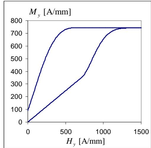
Figure 7. Y-COMPONENT OF THE PREDICTED MAGNETIZATION AT THE COMPRESSIVE STRESS OF 2 MPa.
