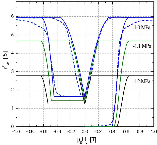
Figure 1. PREDICTED MFIS HYSTERESIS CURVES AT DIFFERENT STRESS LEVELS. SOLID LINES: MODEL, DASHED LINE: EXPERIMENTAL DATA [2].
