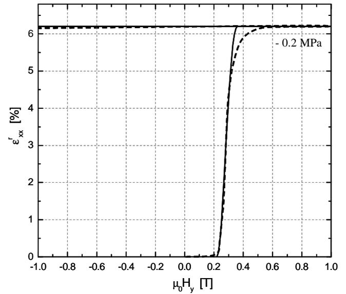
Figure 3. PREDICTED MFIS HYSTERESIS CURVE. SOLID LINES: MODEL, DASHED LINE: EXPERIMENTAL DATA [2].
