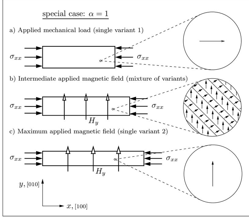
**Figure 2.** Special loading case for the magnetic field-induced variant rearrangement process.
