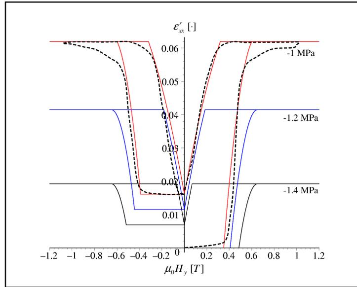
**Figure 3.** Axial reorientation strain vs. transversely applied magnetic field for different bias stress levels. Numerical results—solid lines, experimental data (-1.0 MPa)—dashed line.
