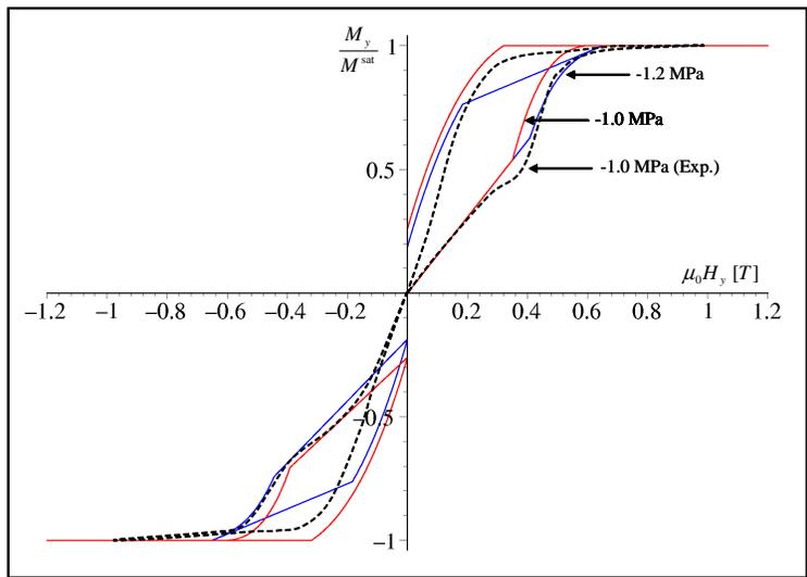
**Figure 5.** Transverse magnetization vs. transversely applied magnetic field for different bias stress levels. Numerical results—solid lines, experimental data ( $-1.0$  MPa)—dashed line.
