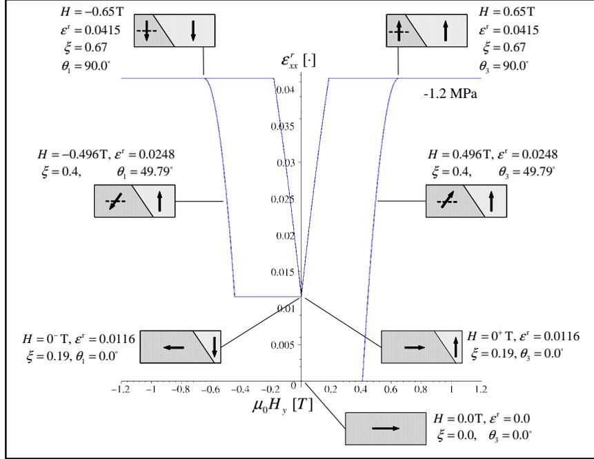
**Figure 4.** Schematic illustration of the evolution of the variant volume fraction and the magnetization rotation for the predicted hysteresis loop under  $-1.2$  MPa.
