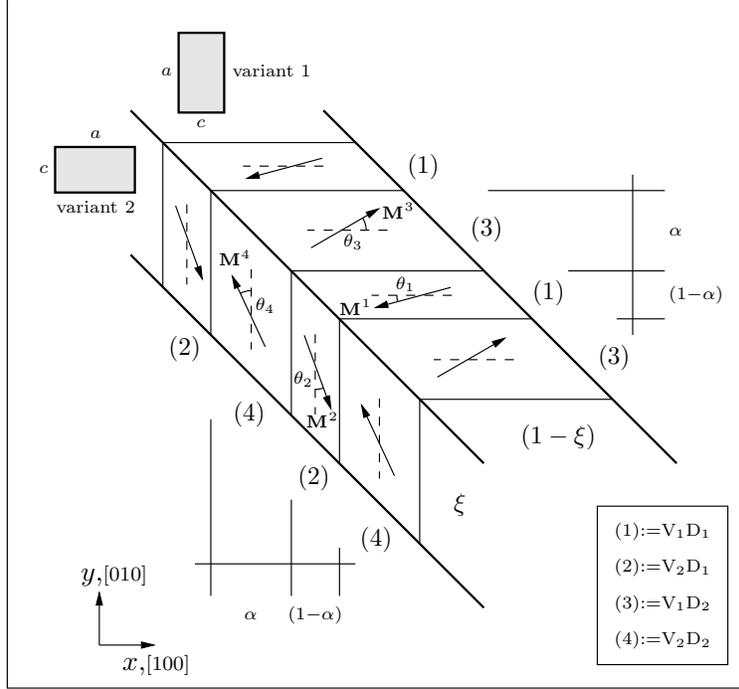
**Figure 1.** Coexistence of martensitic variants and magnetic domains at a twin boundary during the variant reorientation process. The angles  $\theta_i$  measure the rotation of magnetization vectors with respect to the magnetic easy axes. The four distinct domains are numbered 1–4 to simplify the notation. The abbreviation  $V_1 D_2$ , for example, stands for "variant 1, domain 2".
