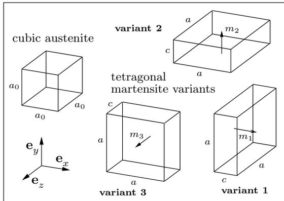
(b) Crystal structure of the austenite phase and the martensite variants. The magnetization per unit volume within each martensitic unit cell is denoted  $m_i$ .
