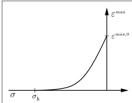
**Figure 5.** Schematic of the approximated dependence of the maximum reorientation strain on the applied axial stress.
