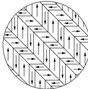
(c) Martensitic variant and magnetic domain structure at intermediate applied magnetic fields.
