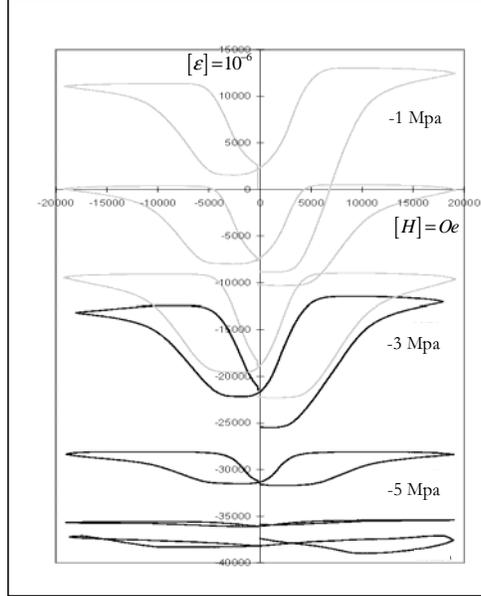
**Figure 1.** Strain vs. magnetic field behavior of NiMnGa single crystal specimen under different constant stress levels as reported by Tickle.<sup>4,5</sup>
