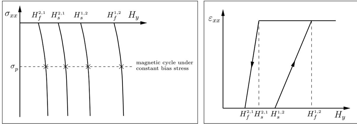
(a) Phase diagram for the variant reorientation process in MSMA. Displayed are the reorientation start and finish lines for the forward and reverse directions, respectively.
