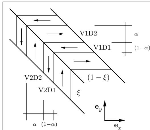
**Figure 3.** Coexistence of martensitic variants and magnetic domains at a twin boundary during the reorientation process.
