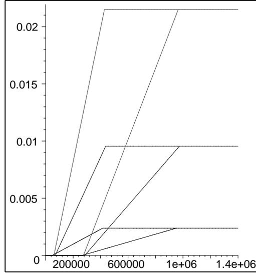
**Figure 6.** Axial reorientation strain vs. transversely applied magnetic field [ $\text{Am}^{-1}$ ] for NiMnGa specimen at bias stress levels of  $-1$  MPa,  $-3$  MPa and  $-5$  MPa.
