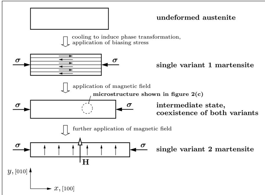
(a) Schematic of experimental setup used for the NiMnGa single crystal measurements of axial strain vs. transverse magnetic field starting from a single martensitic variant state (cf. Tickle<sup>3,4</sup>).
