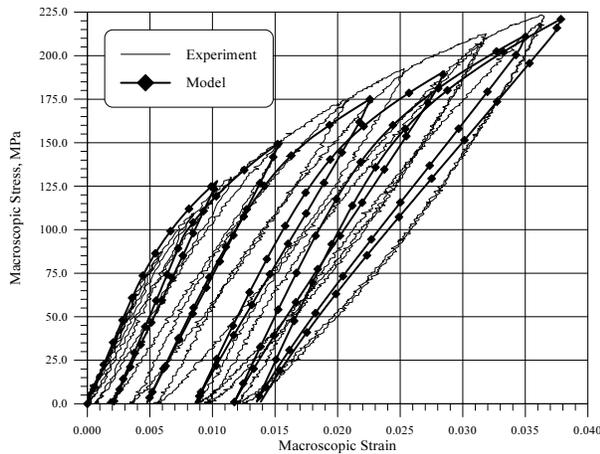
**Figure 6.** Stress-strain response of a large pore porous NiTi SMA bar — comparison between the experimental results and the model simulation.
