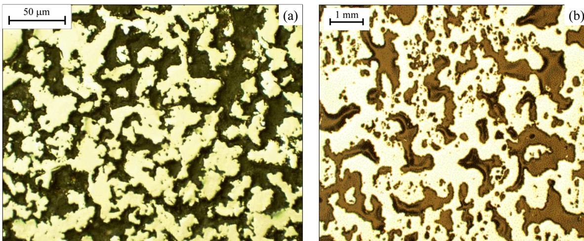
**Figure 1:** Microphotograph of porous NiTi specimens: (a) small pore specimen; (b) large pore specimen.
