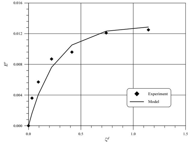
**Figure 7.** Plastic strain  $E^p$  versus accumulated detwinned martensitic volume fraction  $\zeta^d$  for the large pore porous NiTi.
