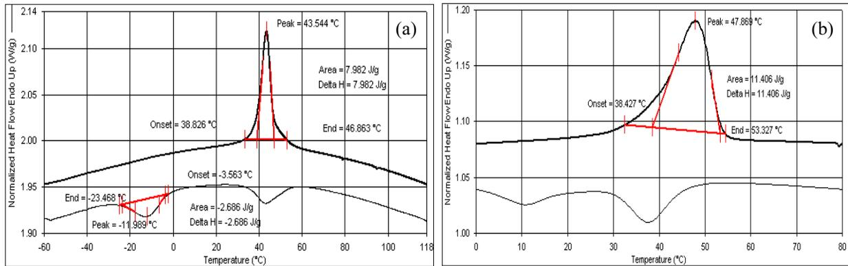
**Figure 2:** DSC results for porous NiTi: (a) small pore alloy; (b) large pore alloy.
