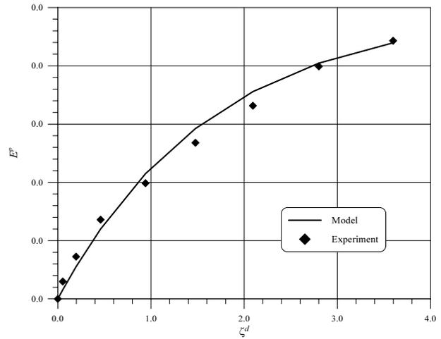
**Figure 5.** Plastic strain  $E^p$  versus accumulated detwinned martensitic volume fraction  $\zeta^d$  for the small pore porous NiTi.
