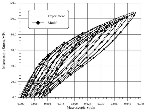
**Figure 4.** Stress-strain response of a small pore porous NiTi SMA bar — comparison between the experimental results and the model simulation.
