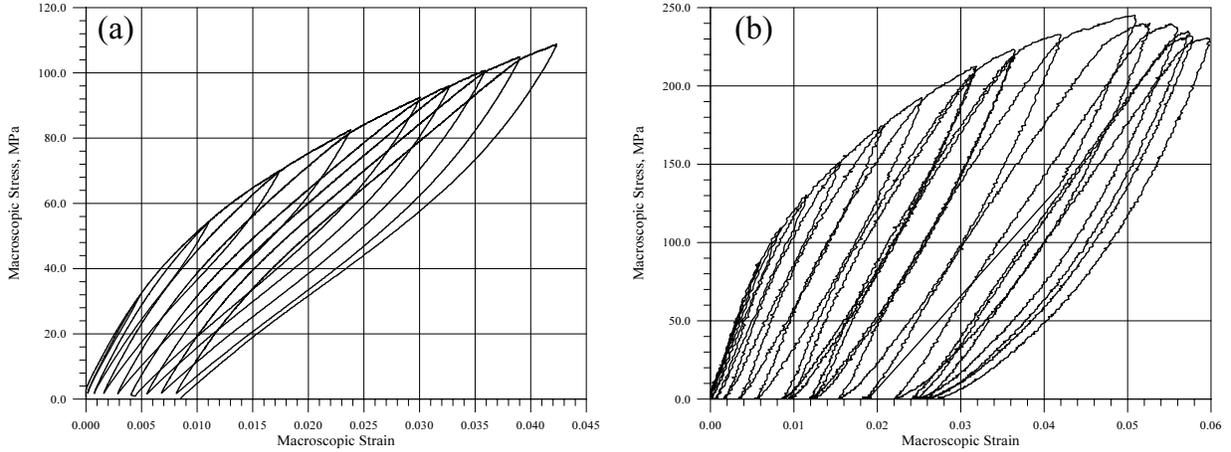
**Figure 3:** Stress-strain response of porous NiTi tested at 60°C: (a) small pore alloy; (b) large pore alloy.
