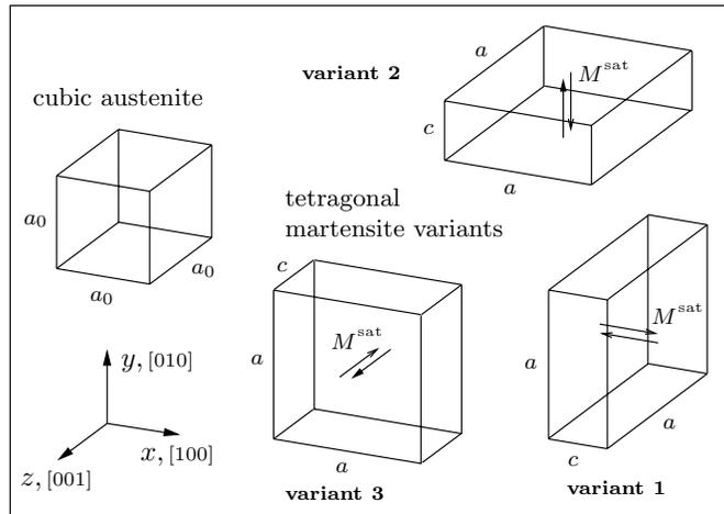
Figure 1: Crystal structure of the austenitic phase and the tetragonal martensite variants in NiMnGa. Arrows indicate the possible orientations of the saturation magnetization  $M^{\text{sat}}$  within each variant.
