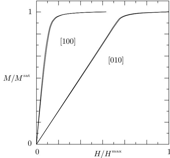
Figure 7: Qualitative magnetization curves of the single variant MSMA specimen magnetized along the compression and perpendicular axes. For quantitative experimental results cf. Tickle and James (1999).
