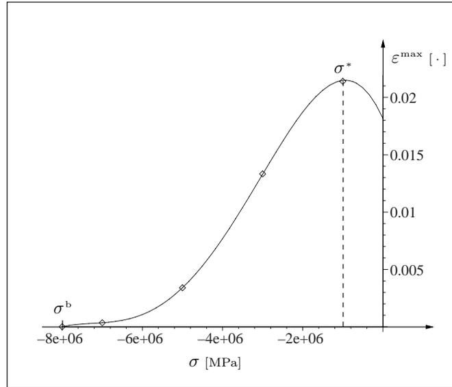
Figure 10: Stress dependence of the maximum magnetically induced reorientation strain. Shown are experimental data (Tickle, 2000) corresponding to different bias stress values (diamonds), and the approximated functional dependence used in the numerical example (solid line).
