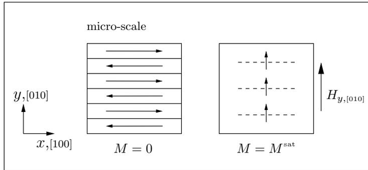
Figure 6: Magnetization of the single variant specimen perpendicular to the compression axis (hard axis).
