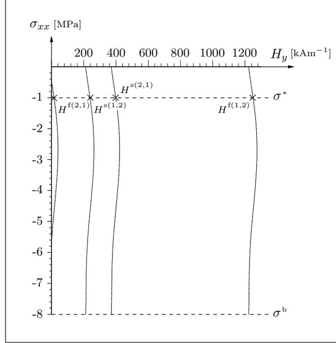
Figure 11: Numerical phase diagram for the variant reorientation process in the  $\text{Ni}_2\text{MnGa}$  alloy specified in Table 2. Displayed are the reorientation start and finish surfaces for the forward and reverse direction, respectively.
