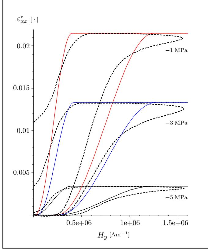
Figure 13: Comparison of the trigonometric hardening model curves (solid lines) and the experimental data (dashed lines) reported by Tickle (2000).
