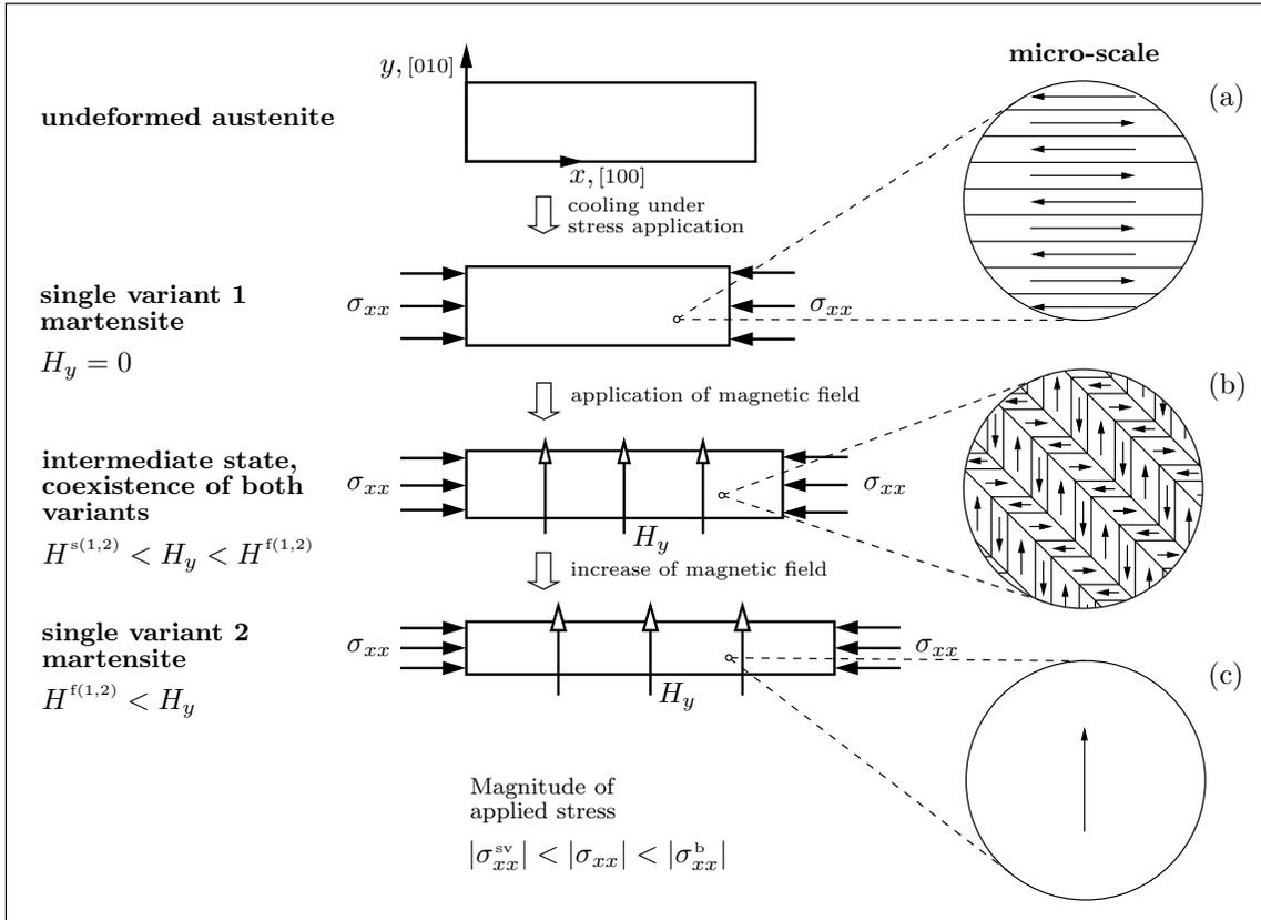
Figure 2: Schematic of several configurations of a NiMnGa single crystal specimen, corresponding to increasing applied magnetic field levels, as observed in an experiment devised to measure the strain vs. magnetic field response of NiMnGa under a constant compressive mechanical load (Tickle and James, 1999; Tickle, 2000). Additionally, Schematics (a)–(c) depict the respective magnetic and crystallographic microstructural arrangements of martensitic variants and magnetic domains.
