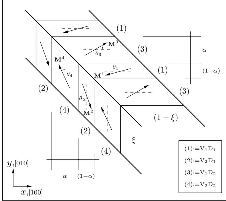
Figure 8: Coexistence of martensitic variants and magnetic domains at a twin boundary during the reorientation process. The angles  $\theta_i$  represent the rotation of magnetization vectors (solid arrows) with respect to the magnetic easy axes along which they are oriented in their reference configurations (dashed arrows). The abbreviation  $V_1 D_2$ , for example, stands for "variant 1, domain 2". The four distinct subdomains are numbered 1–4 to simplify the notation.
