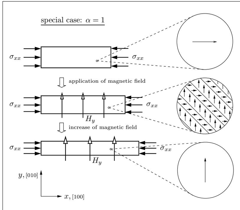
Figure 9: The variant reorientation process with fixed domain structure  $\alpha = 1$ .
