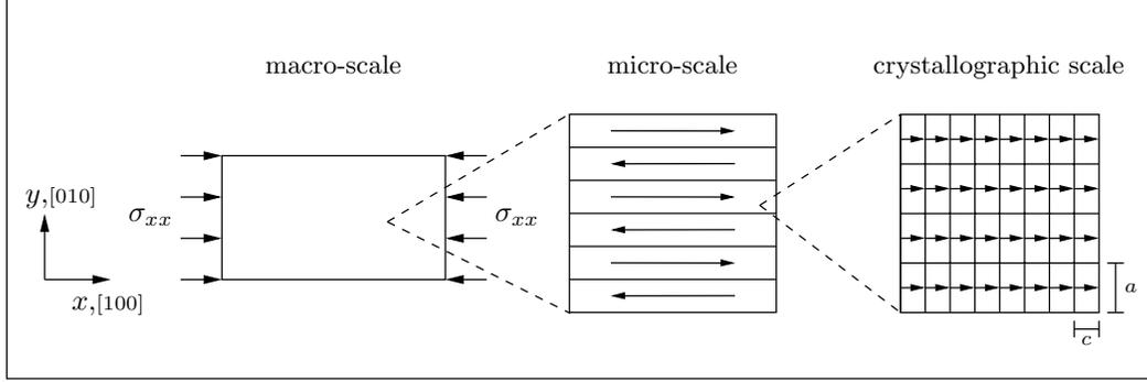
Figure 4: A schematic of the initial single variant 1 martensite state. The variant reorientation is suppressed by an axial compressive stress higher than the blocking stress. Also shown, schematics of the corresponding microscopic scale and the crystallographic scale.
