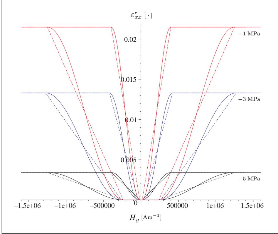
Figure 12: Axial reorientation strain vs. transverse magnetic field for different bias stress levels. Compared are the polynomial (dashed lines) and trigonometric (solid lines) hardening model predictions.
