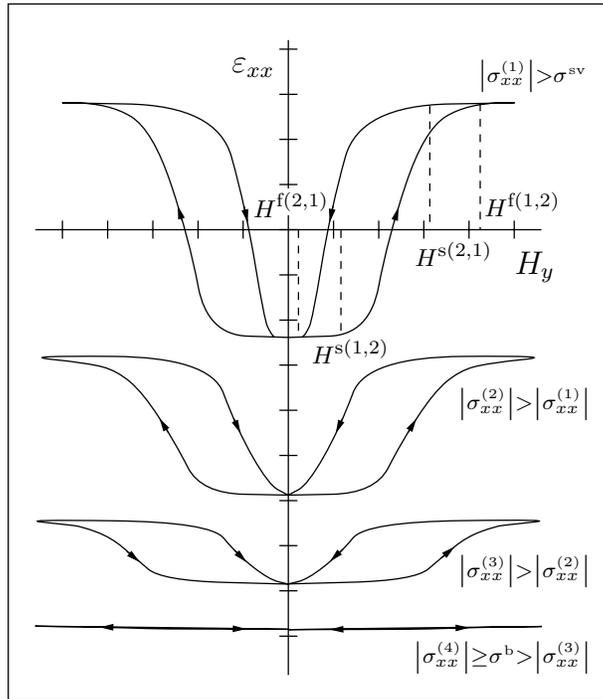
Figure 3: Schematic strain vs. magnetic field response of a MSMA single crystal for different axial bias stress levels.
