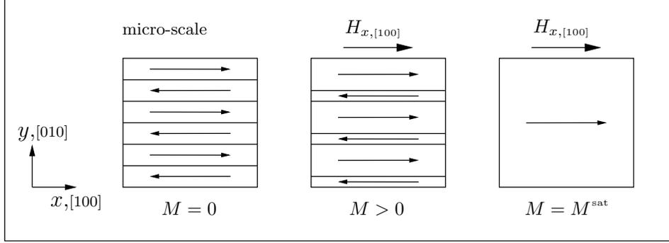
Figure 5: Magnetization of the single variant specimen along the compression axis (easy axis).
