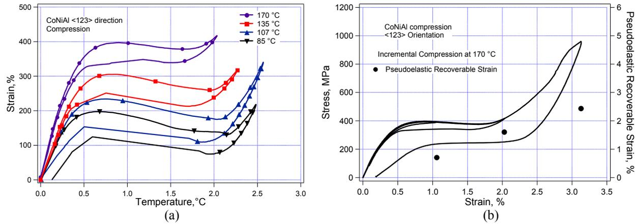
**Figure 5:** a) The temperature and b) the strain dependence of the pseudoelastic response of the [123] orientation.
