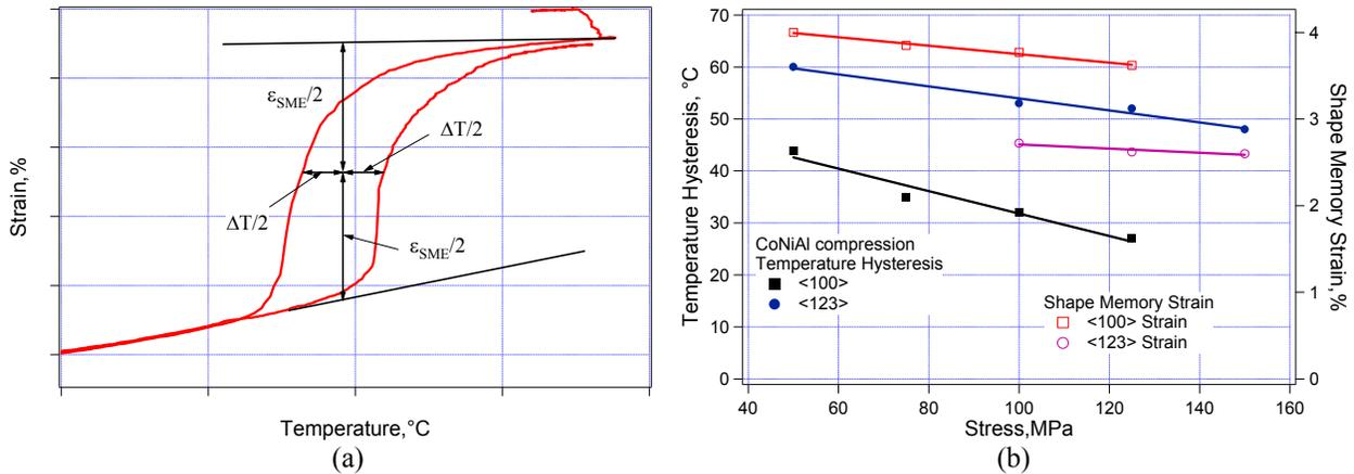
**Figure 3:** a) A schematic for the definitions of the temperature hysteresis ( $\Delta T$ ) and shape memory strain ( $\epsilon_{SME}$ ), b) Change in  $\Delta T$  and  $\epsilon_{SME}$  as a function of applied stress along different orientations.
