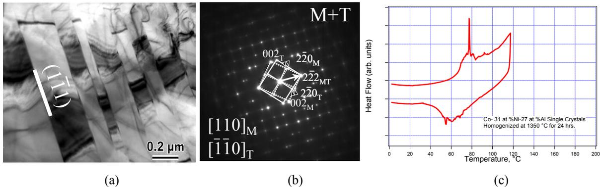
**Figure 1.** a) Bright field TEM image and b) the corresponding diffraction pattern of the present alloy. (c) DSC response after homogenization and water quenching. The internal twinning plane is determined to be  $(1\bar{1}1)$ . M: martensite, T: internal twin.
