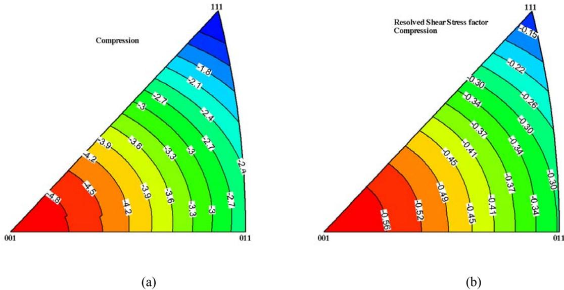
**Figure 6.** Transformation strain (a) and resolved shear stress factor (b) contours for the B2 to L1<sub>0</sub> phase transformation in the present alloy under compression.
