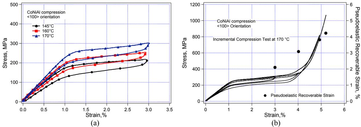
**Figure 4:** a) The temperature and b) strain dependence of the pseudoelastic response of the [100] orientation.
