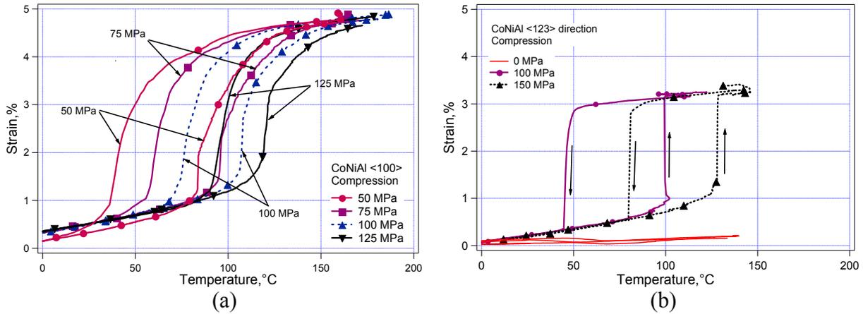
**Figure 2:** Strain vs. temperature response of the a) [100] and b) [123] orientations under constant compressive stress.
