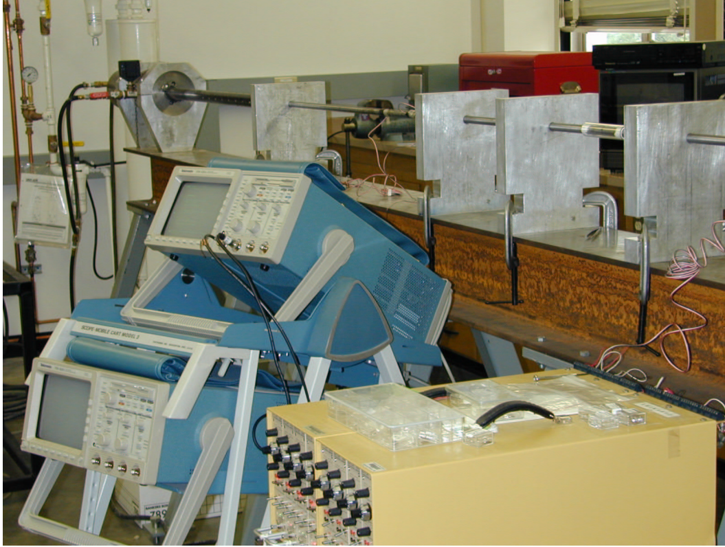
Fig. 11. Photograph of the Hopkinson bar experimental setup. The specimen is visible at the top-right part of the photograph
