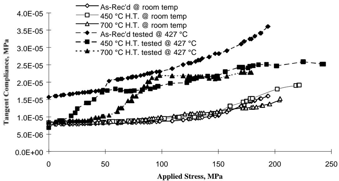
Fig. 15 Instantaneous plastic compliance vs. applied stress for simulation of plastic stress/strain evolution.
