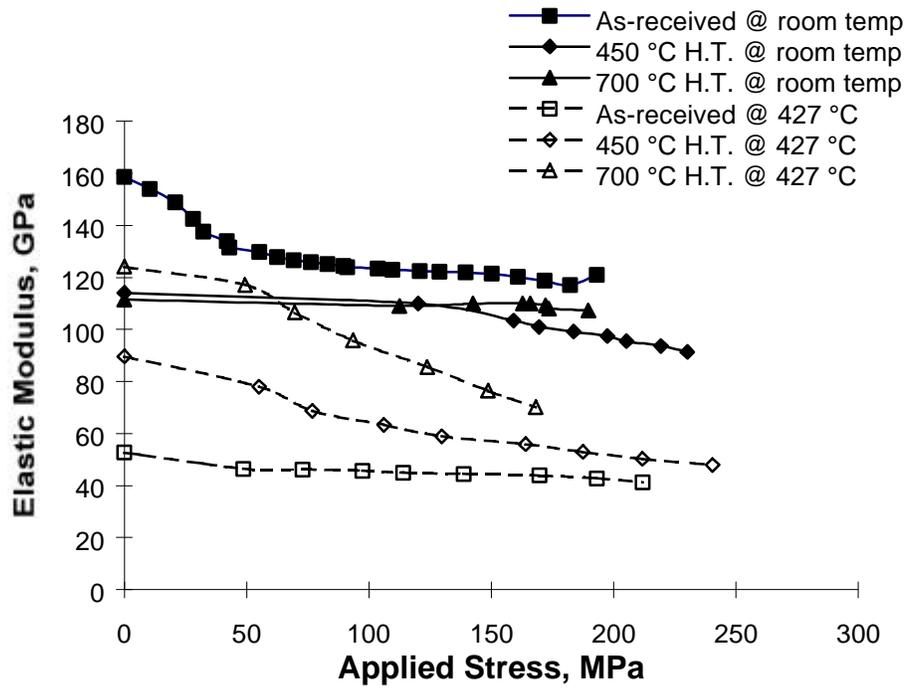
Fig. 11 Unloading Elastic Modulus vs. Applied Stress for transverse specimens.
