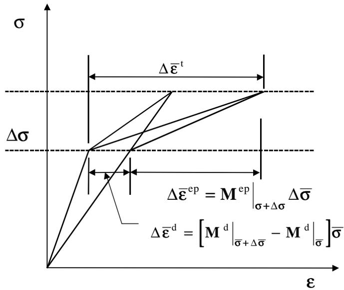
Fig. 13 Schematic representation of uni-axial loading path showing damage and plastic strain increments over loading increment,  $\Delta\sigma$ .
