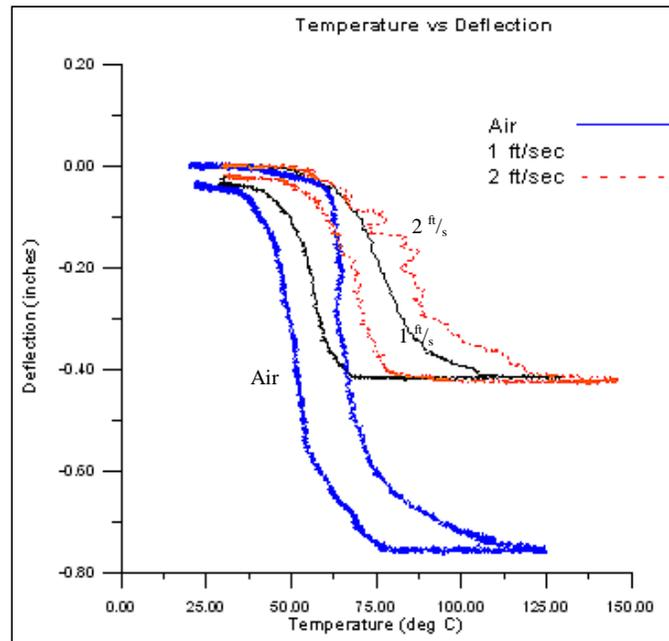
Figure 8. Hydrofoil experimental test results comparing trailing edge deflection vs., wire temperature of hydrofoil in air and in water tunnel at two fluid velocities.
