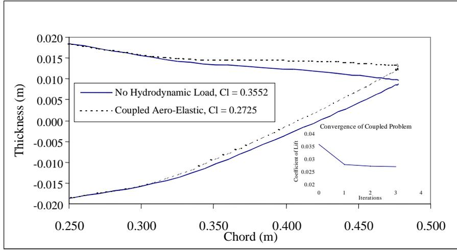
Figure 6. Hydrofoil trailing edge deflection showing the effect of hydrodynamic forces and rate of convergence of the iterative coupling scheme.
