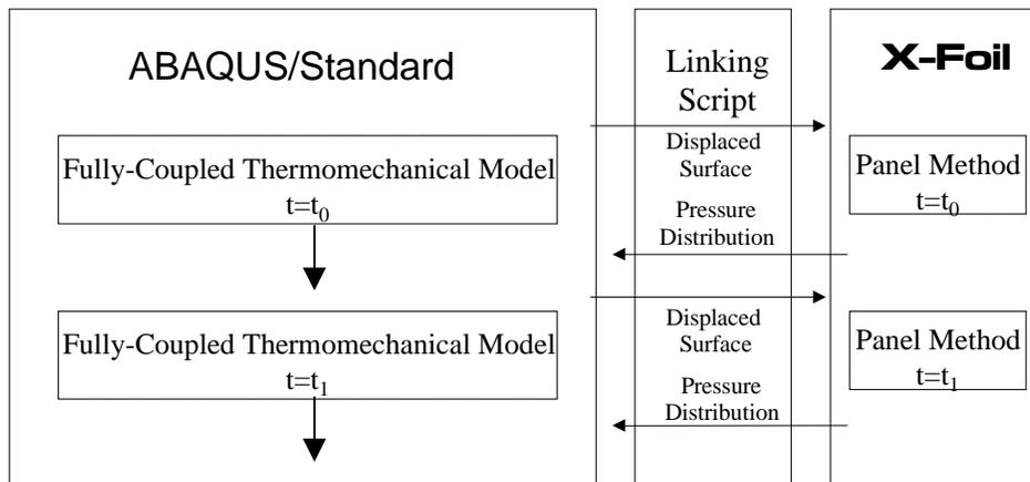
Figure 5. Schematic of hydro-mechanical coupling procedure.
