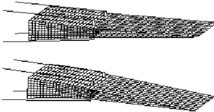
Figure 4. Finite Element mesh of hydrofoil trailing edge and the deformed mesh at maximum deflection.
