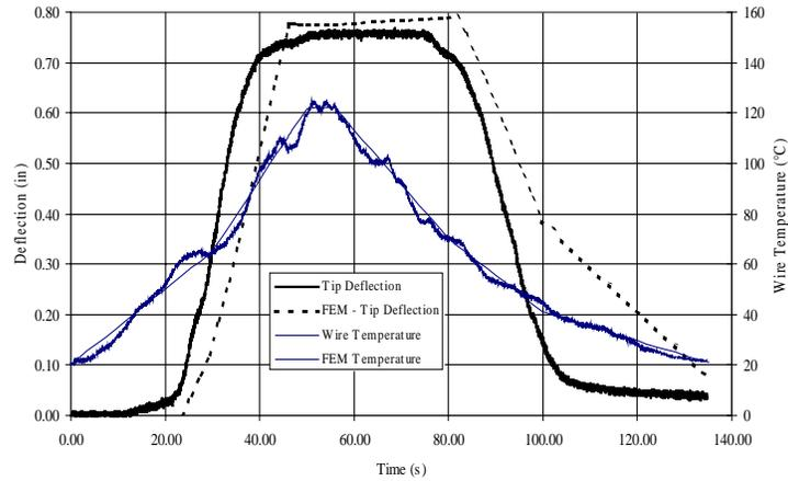
Figure 7. Experimental and numerical hydrofoil (trailing edge) tip deflection and wire temperature versus time for quasi-static actuation in still air.
