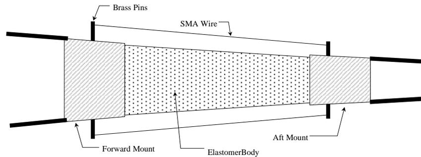
Figure 1. Schematic of hydrofoil center section
