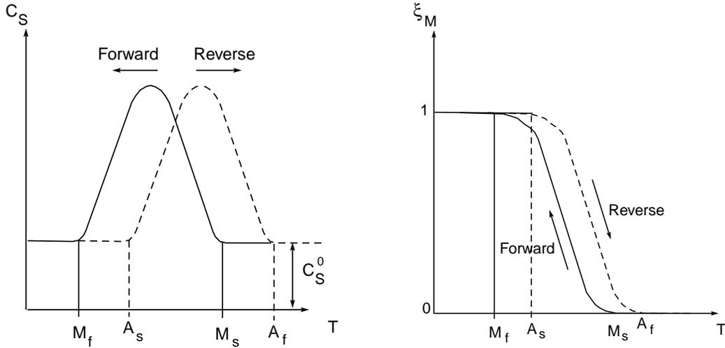
Figure 3: (a) Schematic dependence of  $C_S$  on temperature and (b) the evolution of martensite volume fraction,  $\xi_M$ , during the forward and reverse transformations.
