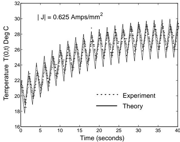
Figure 16: Comparison of the cyclic thermal response between experiment and prediction, for copper with thickness,  $d_s = 4$  mm.
