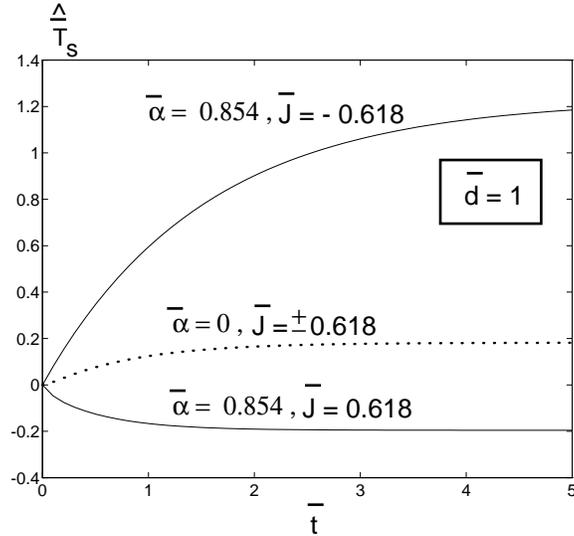
Figure 4: Influence of the directional effect of the current density,  $\bar{J}$ , on heating and cooling of the SMA.
