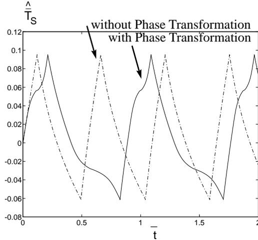
Figure 8: Comparison of the cyclic cooling curves of a SMA undergoing a phase transformation with one without a phase transformation.
