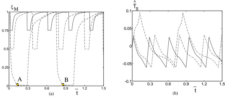
Figure 9: (a) Change in volume fraction of martensite and (b) cyclic temperature profile of SMA with partial and full transformation.
