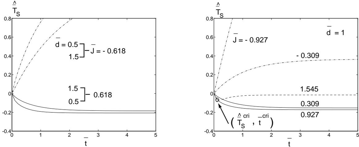
Figure 5: Influence of (a) length,  $\bar{d}$ , and (b) the current density,  $\bar{J}$  on the heating and cooling of the SMA.
