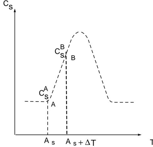
Figure 7: Schematic depiction of the changing heat capacity of the SMA during the phase transformation and its incorporation in the heat conduction problem.
