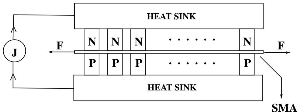
Figure 1: A Proposed SMA actuator
